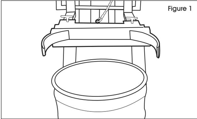
2. Slowly lower the forks to position the drum grabber clamps in the center of the drum, stopping just below the raised ring. (See Figure 2)
