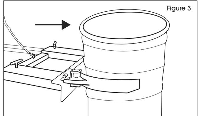
4. Lift the forks and the drum will be clamped and lifted. Carry the drum to the desired destination.
