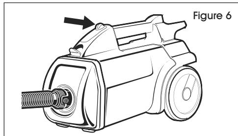
2. Press with hand or foot once to turn on. Press again to shut off.
