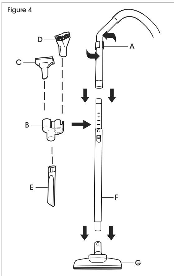
5. Telescopic wand (F) adjusts to different cleaning heights. The combination floor tool (G) works on both carpet and hard surfaces by moving the lever on the floor tool head to either the carpet or bare floor position. (See Figure 4)
