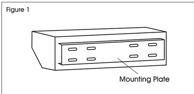
2. Use the mounting plate to determine the mounting location. Fix mounting plate to wall using appropriate fasteners for the mounting surface. (Fasteners not included.)
