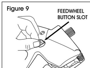
2. Place small coin in feedwheel button slot. (See Figure 9)
