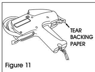
3. Squeeze and release trigger until backing paper is free to be pulled out. (See Figure 11)
