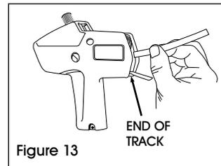
1. With label roll removed, check label track and backing paper track for stray labels.
