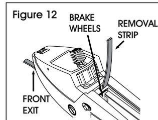
2. Clear label track by squeezing trigger and feeding label removal strip under brake wheels and out front of labeler. (See Figure 12)
