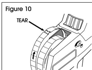
1. Tear label strip at label roll as shown and pull label roll from between hubs. (See Figure 10)
